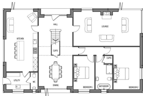
GROUND FLOOR PLAN SCALE 1:100 @ A1
